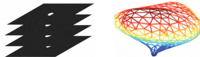
Fig. 1. Generating a 3D mesh for the lung nodule surface from a stack of successive segmented 2D LDCT slices.
